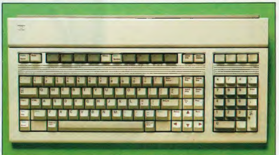
The keyboard is excellent: 107 well laid out keys divided into four functional areas
